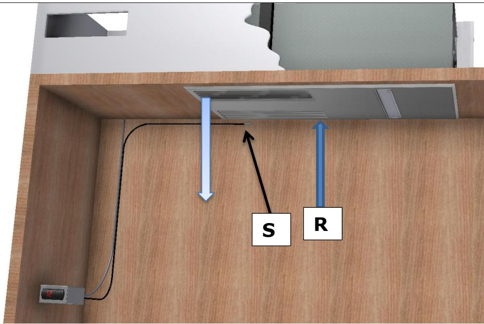
The thermostat can be placed in the cabinet or on the front or outside the cabinet. Its probe (S) must be placed towards the air intake area (R). It is advisable to ensure that the end of the probe does not touch the bulkhead and is in the air flow.
