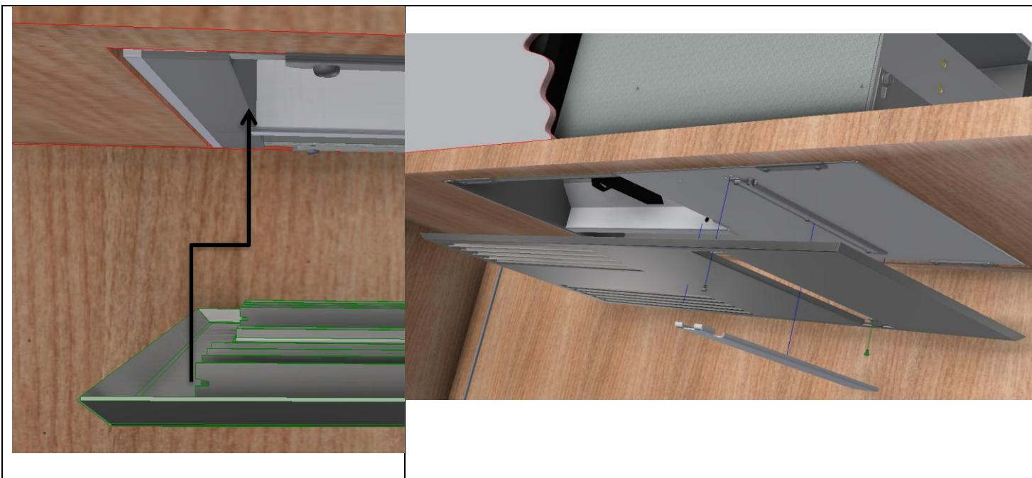
The cover is inserted on the left at the notches and then screwed. The filtre cover is magnetic
