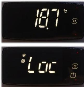
The thermostat is stuck and displays "Loc" if the display is pressed.
