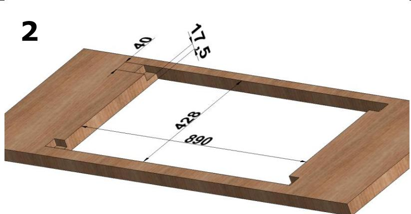
Using the template, trace the location of the air conditioner (be careful that nothing prevents access to the filter hatch)
