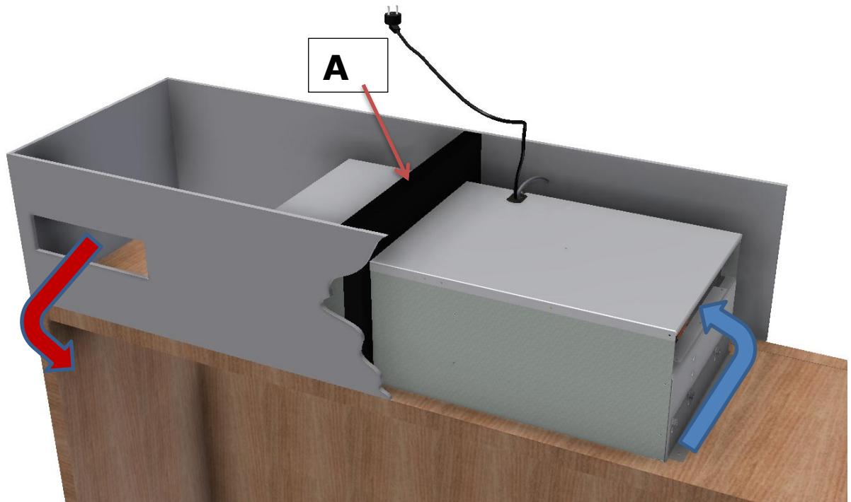
Separate the air flows. The free cross-section of each grid is 200 cm<sup>2</sup>. Separation A is not provided.
